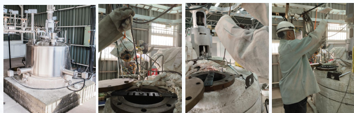
Fig. 2: Procedure for placing and removing samples in a pilot plant.
